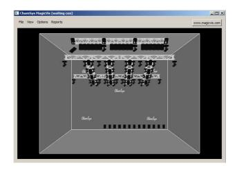
The View Vis tab in the Patch Window will now become visible. Initially the title bar in MagicVis will show "Waiting con". Once a connection has been made with the console then it will change to say "waiting sync". Once the show data has been transferred over the connection from the console to the MagicQ vis application then it will change to say "synced".
