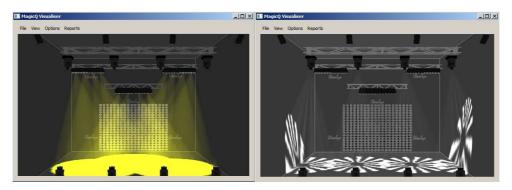
MagicVis is available in two versions. Firstly, a stand alone MagicVis application which can be run on a laptop connected via network to a MagicQ console. Secondly a new version of MagicQ that has the visualiser combined into it for use on PCs and Macs.
