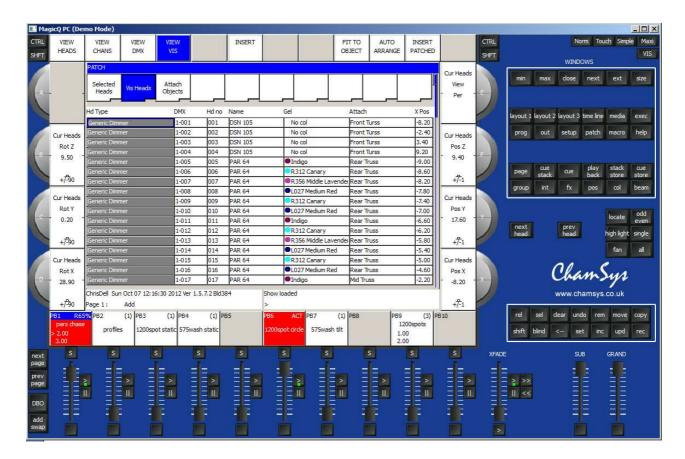
In Selected Heads, all the visualiser heads for the currently selected heads will be shown in the list. Heads are selected as usual using groups or direct from the keypad. In this view the encoders and soft buttons will apply changes to all the visualiser heads for the selected heads.
