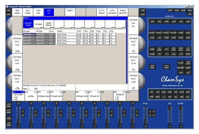
Encoders B, C and D are used for rotation around the X, Y and Z axis.
